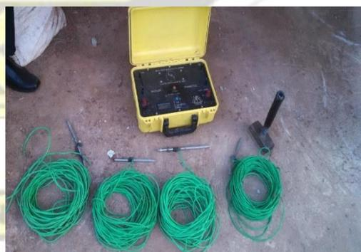
**Figure 3.1b:** Resistivity meter and accessories
