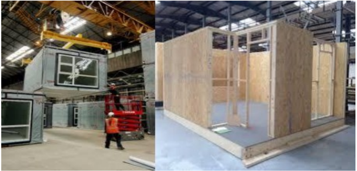
Figure 2.1 Factory producing volumetric units
