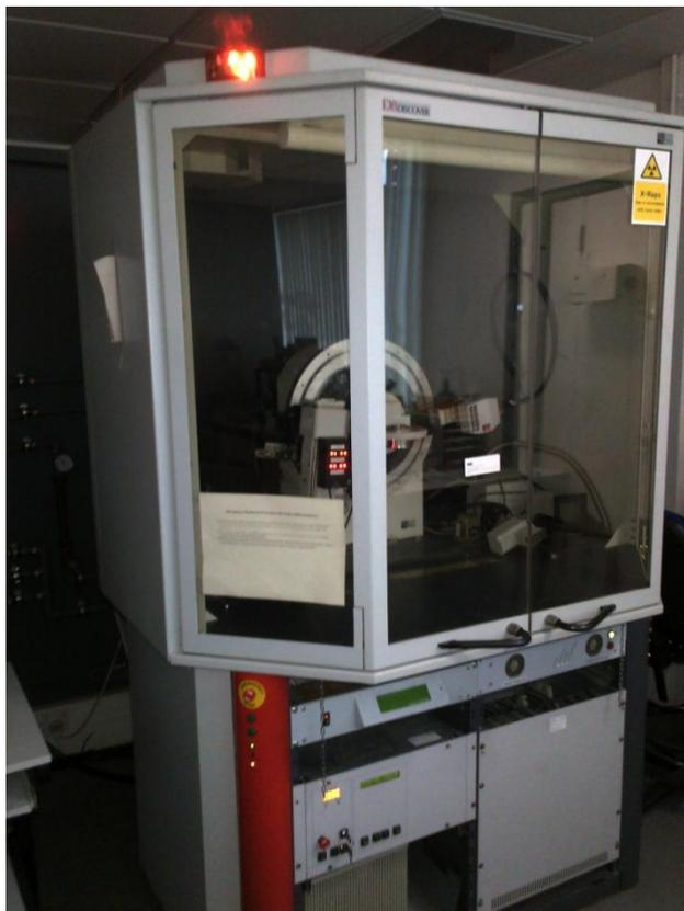
Figure 3.3. A photograph of Bruker AXE D8 Discover X-ray Diffractometer
