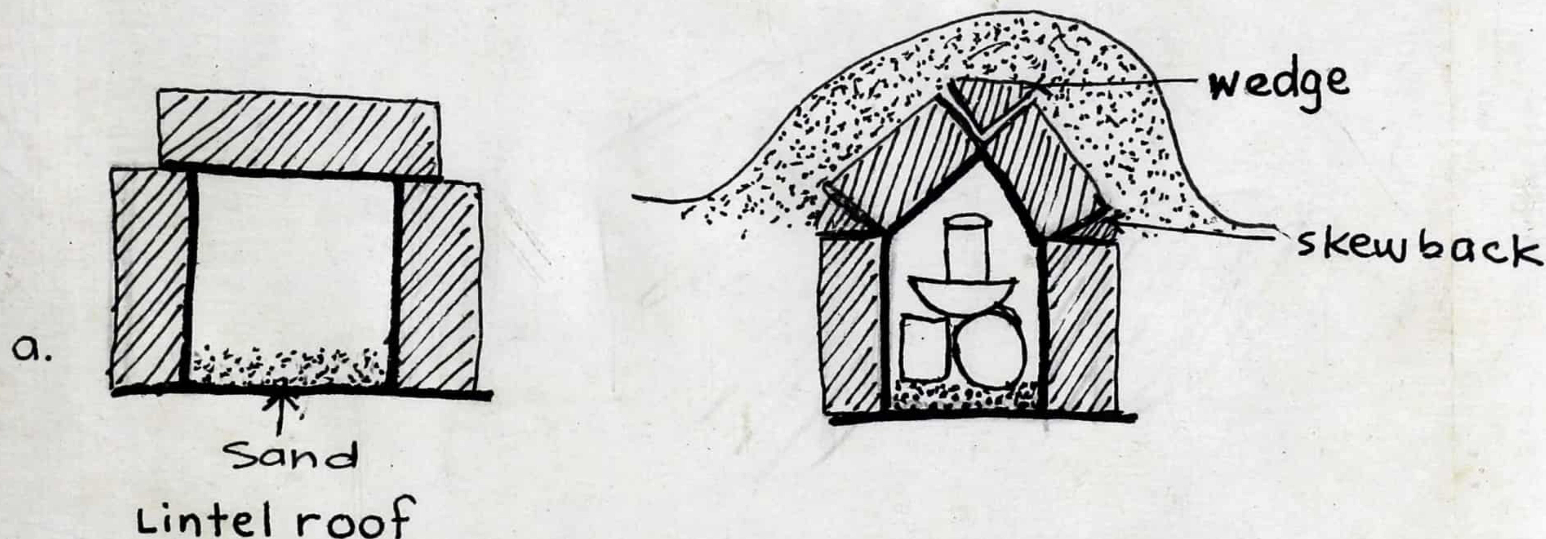
Fig. 11 Roofing a trench kiln.
