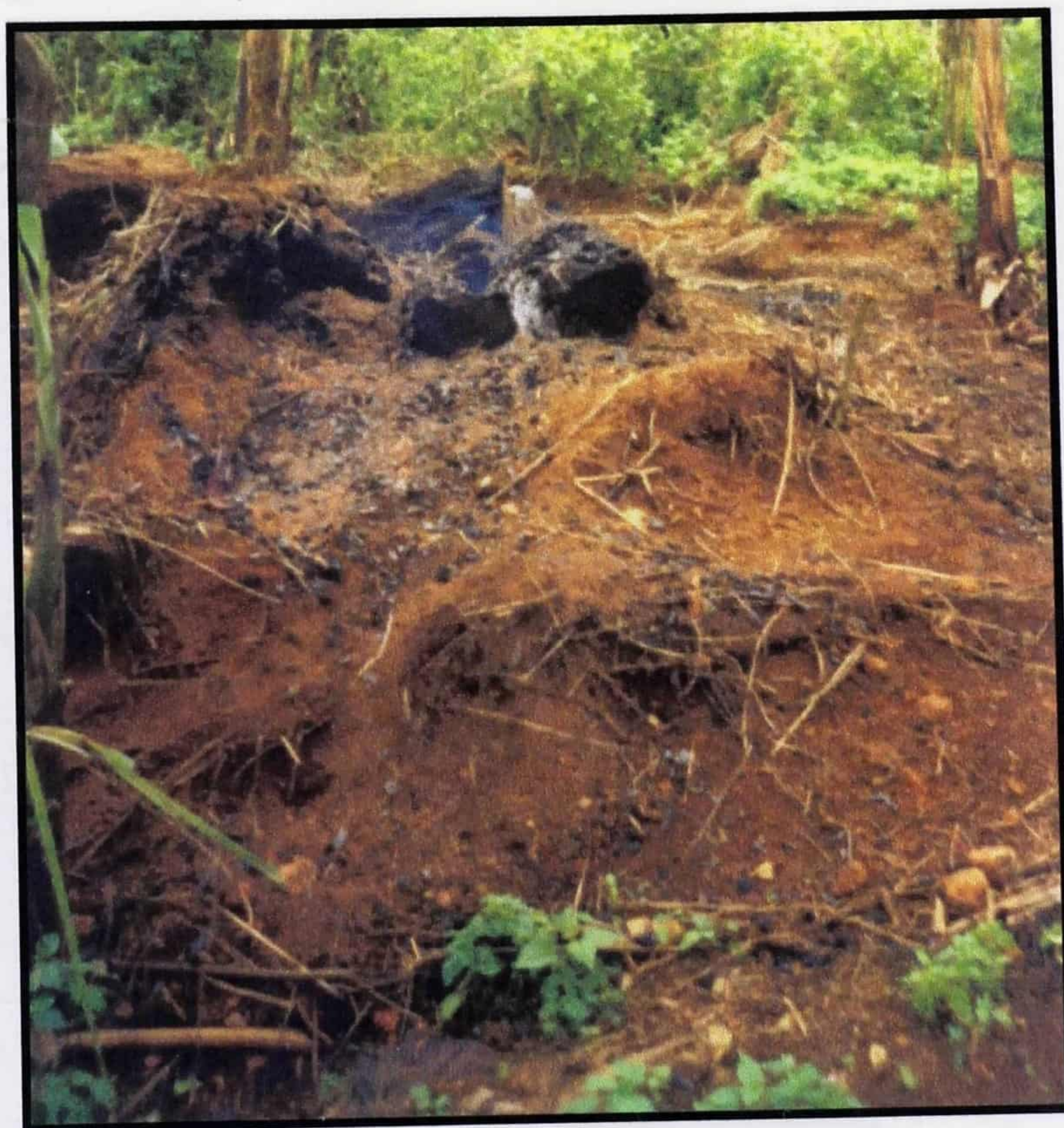
Plate 12. PIT method charcoal production at Antwigyeikrom.
