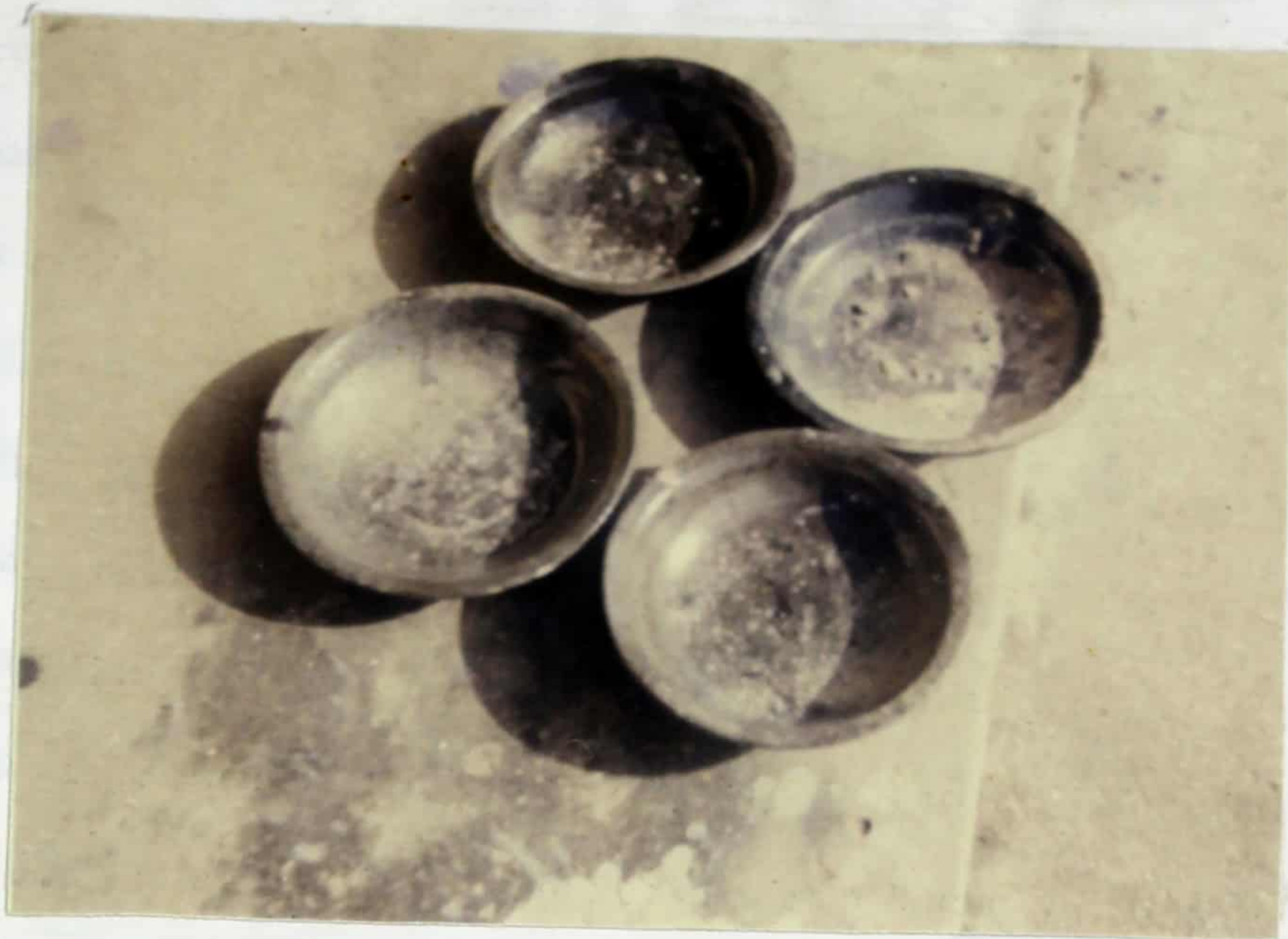
Fig.1 Open bowls spoiled by particles from ceiling of kiln that dropped into them, Winneba Secondary School
