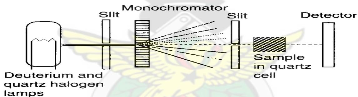
Fig. 8.0 Single beam UV/Vis spectrophotometer
