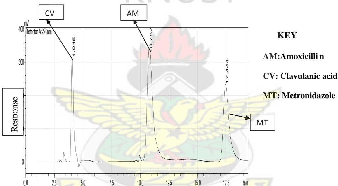
Fig. 19 Chromatogram of Amoxicillin and Clavulanic acid with metronidazole as internal standard
