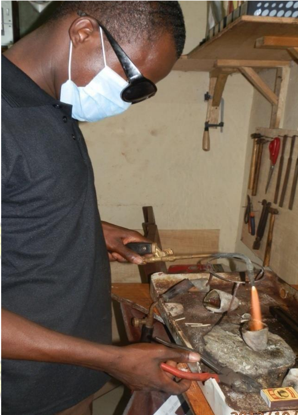
Plate 6. Craftsman melting gold in a crucible.
