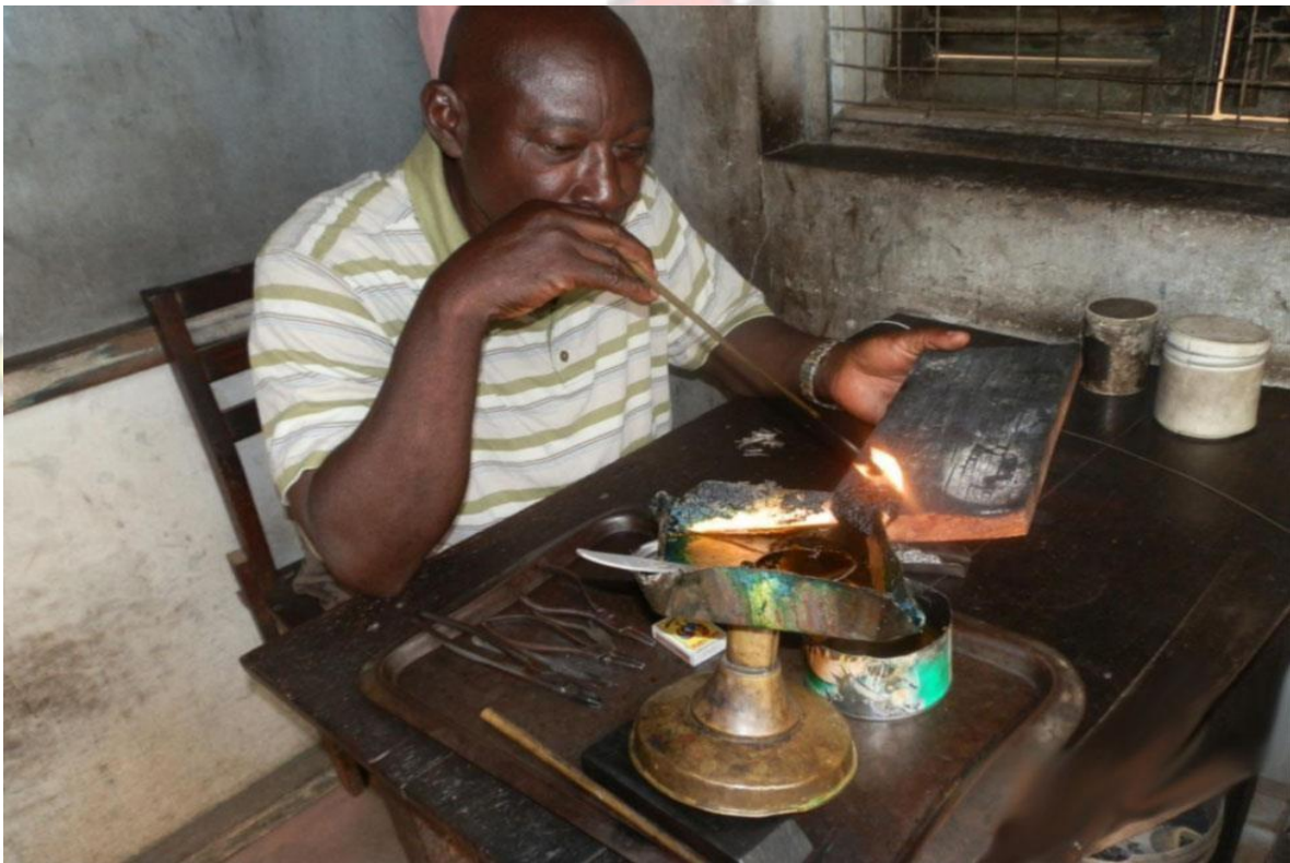
Plate 2. A traditional craftsman soldering with the blow pipe
