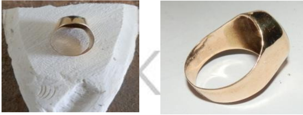
Plate 17. Cuttle fish casting processes
