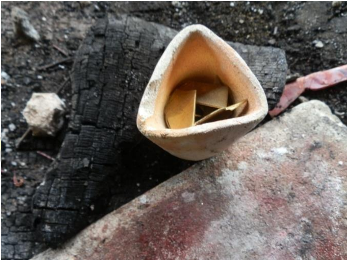
Plate 11. Crucible with gold material
