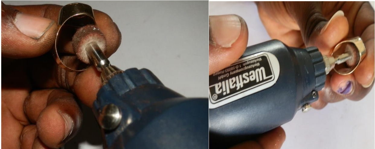
Plate 46. Flexible shaft for polishing intricate and interior parts of objects.
