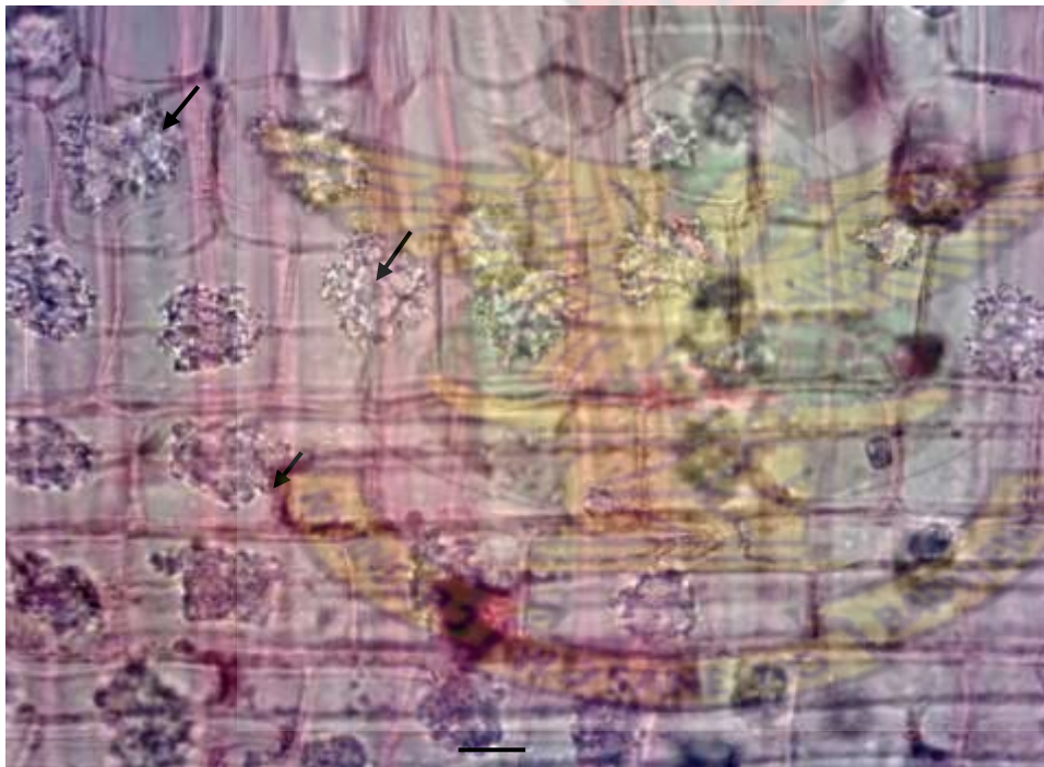
Plate 4.14 Radial-longitudinal section showing Silica bodies (arrowhead) in chambered axial parenchyma
