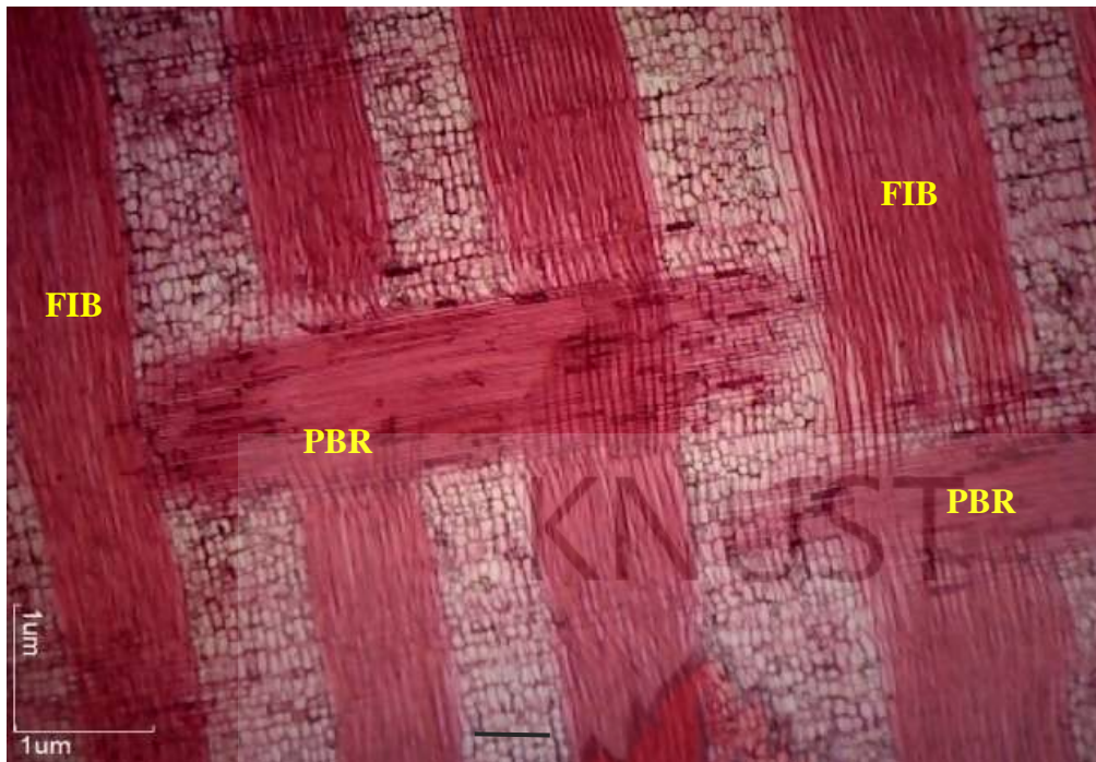
Plate 4.3 Radial-longitudinal section of F. sur showing procumbent ray (PBR) and fibres (FIB)
