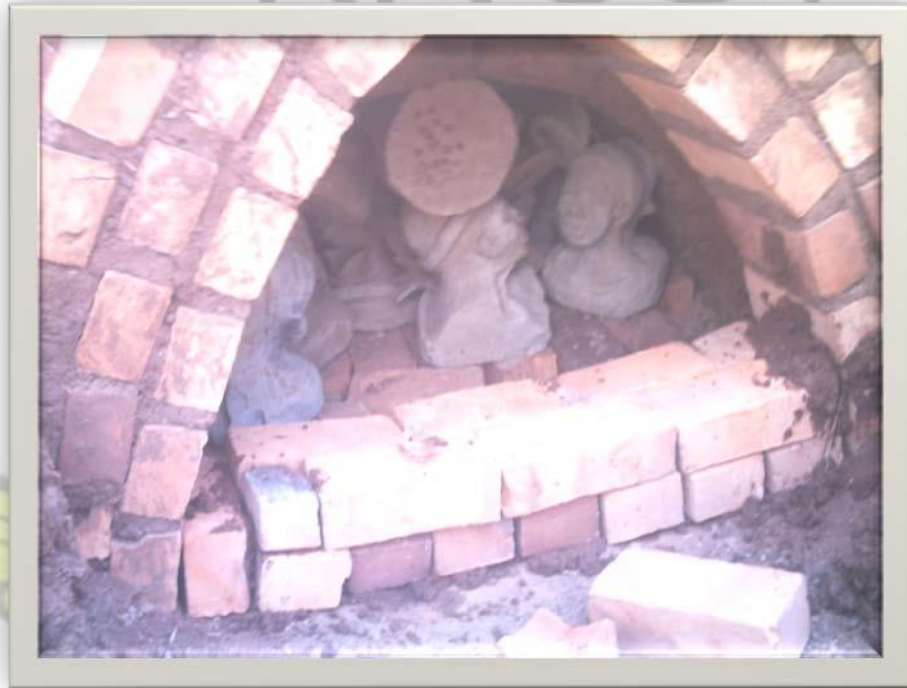
Plate 4.32 Packing the kiln
