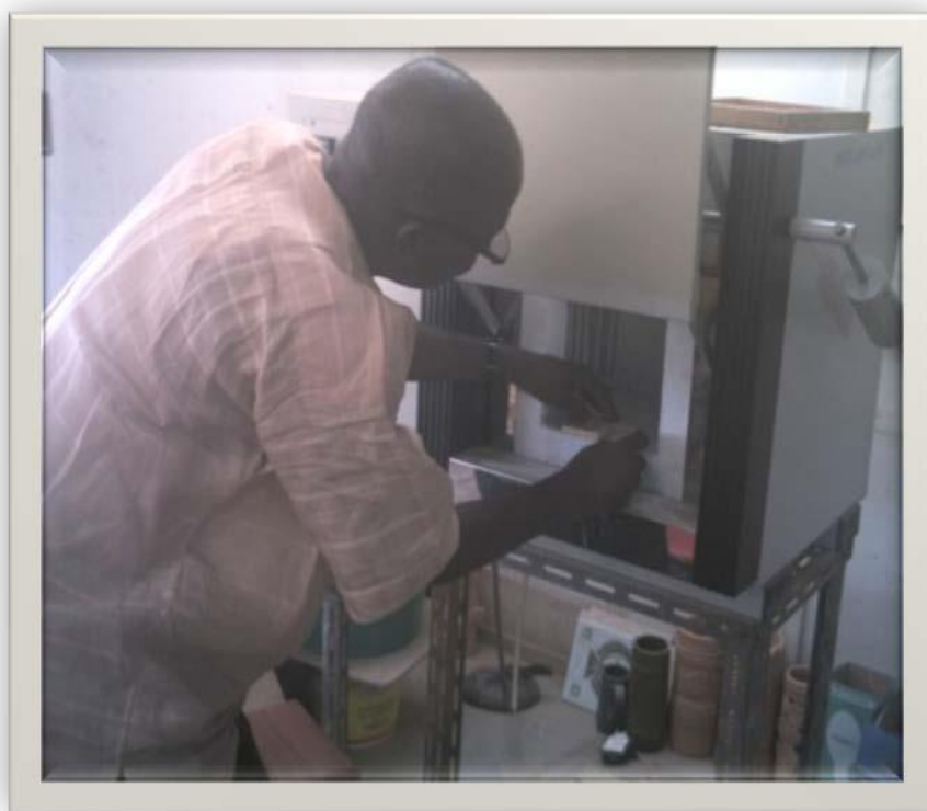
Plate 4.2 Test firing in a test kiln
