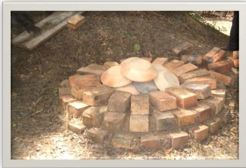
Plate 4.41 Closing the kiln in with bricks
