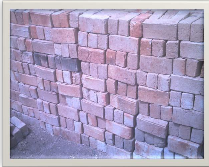
Plate 5.6 Colour variations in fired bricks
