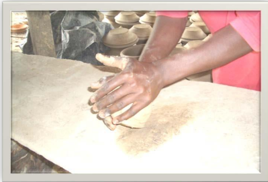
Plate 4.3 Kneading of clay
