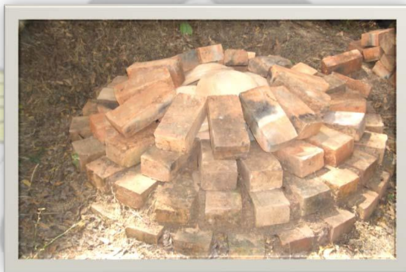
Plate 4.42 Closing the kiln with bricks
