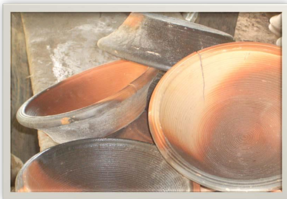
Plate 5.7 Cracks resulting from direct impingement of flames
