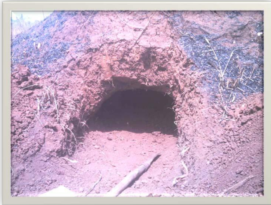
Plate 4.21 Carving out a fire port
