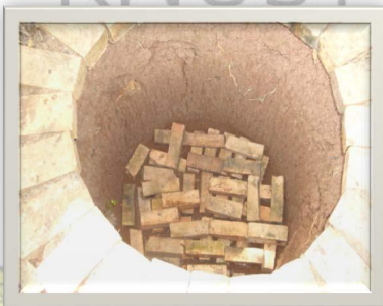
Plate 4.40 Deck prepared to receive wares
