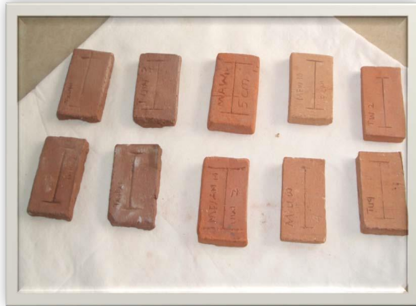
Plate 5.1 Fired colour of the anthill test pieces
