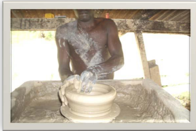
Plate 4.8 Throwing a test piece
