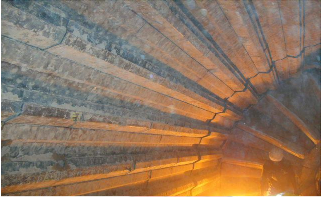
Figure 2.5: Installed rubber and composite liners in a mill
