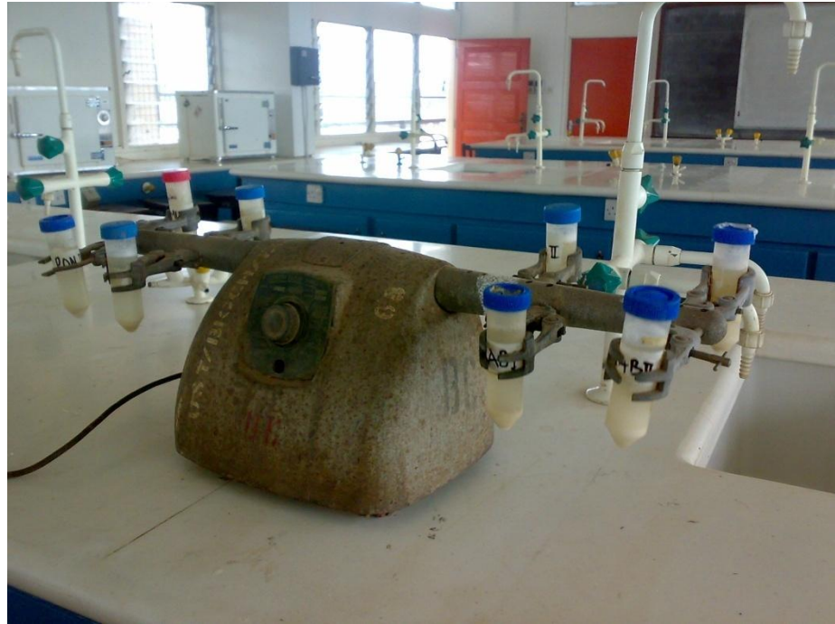
Appendix 8A: Griffin flask shaker being used to agitate samples
