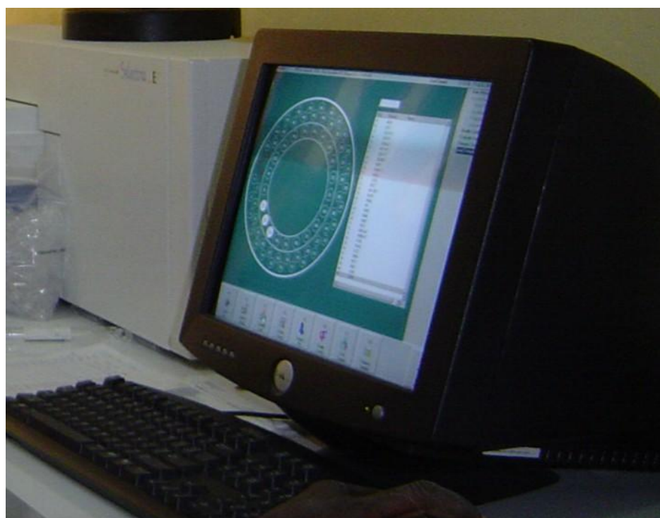
Fig 3.12 Displayed locations of reagent bottles and sample cups on monitor
