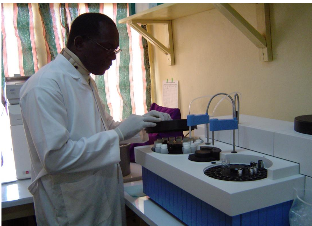
Fig.3.11 Reagent bottles and sample cups arranged in analyzer according to their displayed locations on monitor
