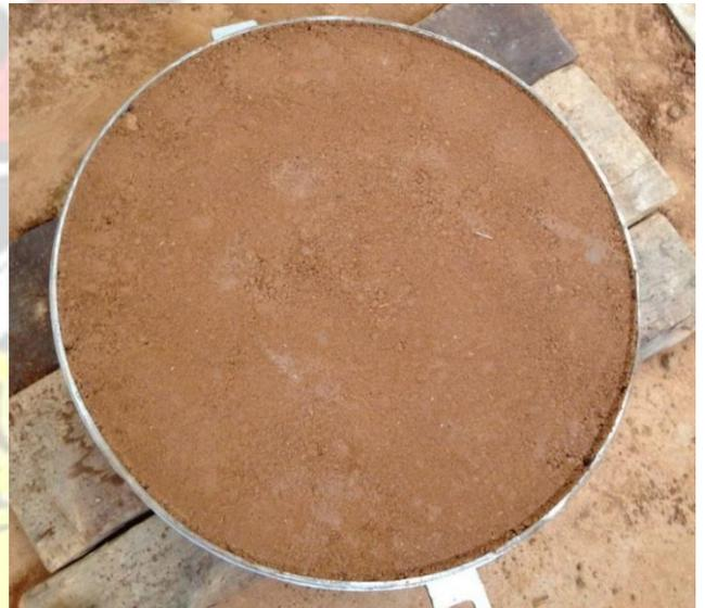
Plate 3.7: Compaction of sample in the mould using the 4.5kg rammer. Plate 3.8: Compacted sample in the mould.
