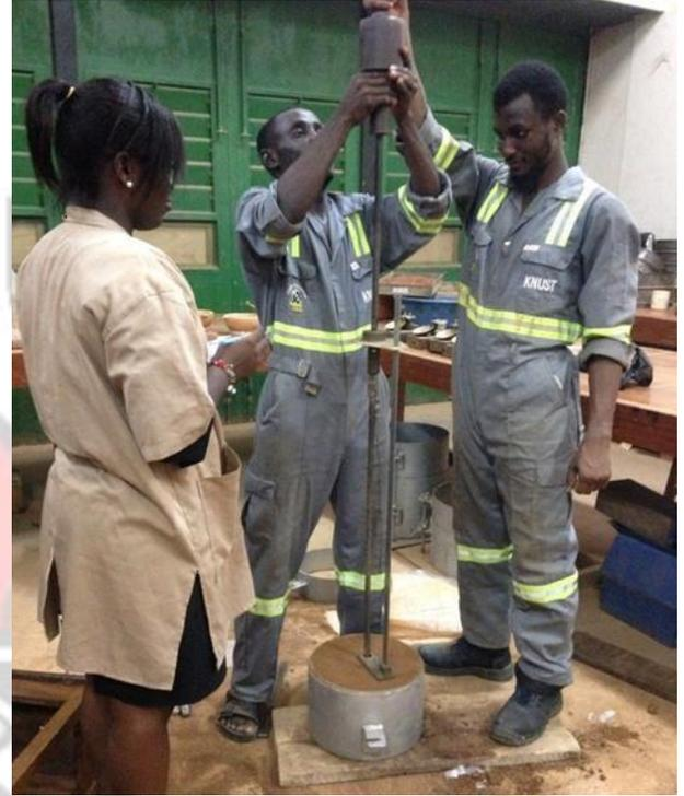
Plate 3.9: Position of the DCP cone centrally on the compacted sample. Plate 3.10: Performing of in-mould DCP test on the compacted sample.
