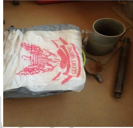
Plate 3.5: Pouring of determined mass of soil Plate 3.6: Covering of remaining in mould to fill a layer of the marked mould portions of soil to preserve height. moisture.
