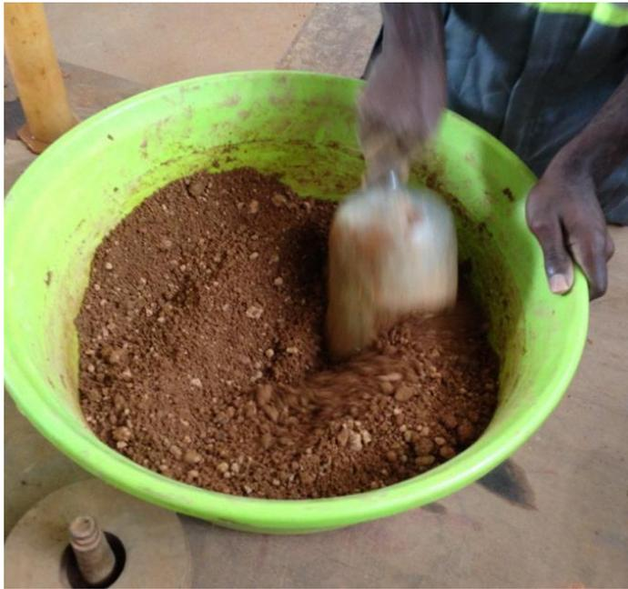
Plate 3.3: Mixing of the lateritic sample.
