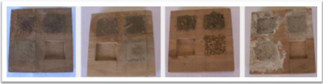
Plate 3.11: Some dry bond ready for abrasion test
