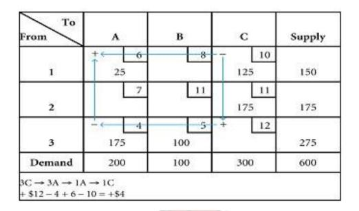
Figure 3.25: The Stepping-Stone Path for Cell 3C
