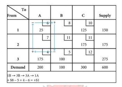
Figure 3.23: The Stepping-Stone Path for Cell 1B
