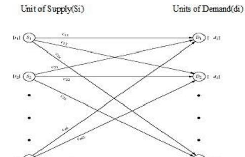
Figure 3.2: Network representation of the transportation problem sources could represent warehouses and the sinks could represent retail.
