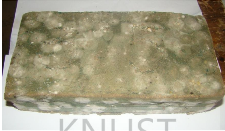
Plate 4.1 Growth of fungus on the drying brick
