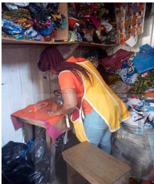
Plate 4.9a: A Master craftsman ironing the collar of a shirt to lie flat.
