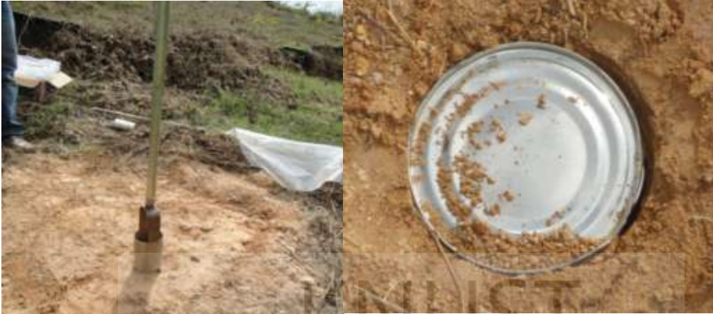
Plate A: Soil sample collection using auger to determine bulk density.
