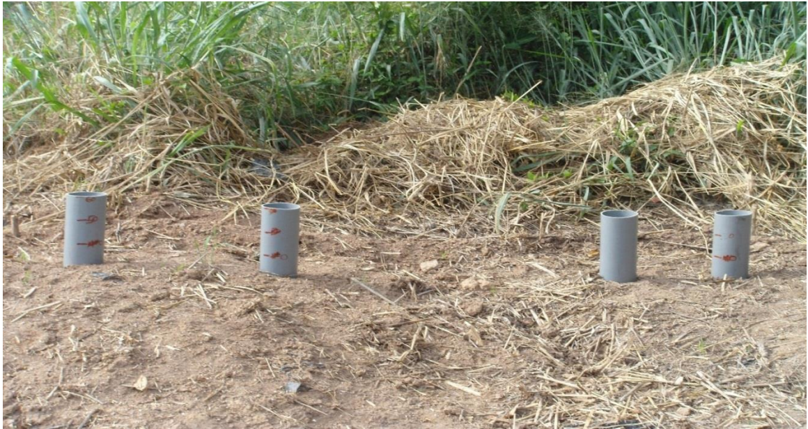
Plate 1: PVC pipes inserted into the soil for sample collection
