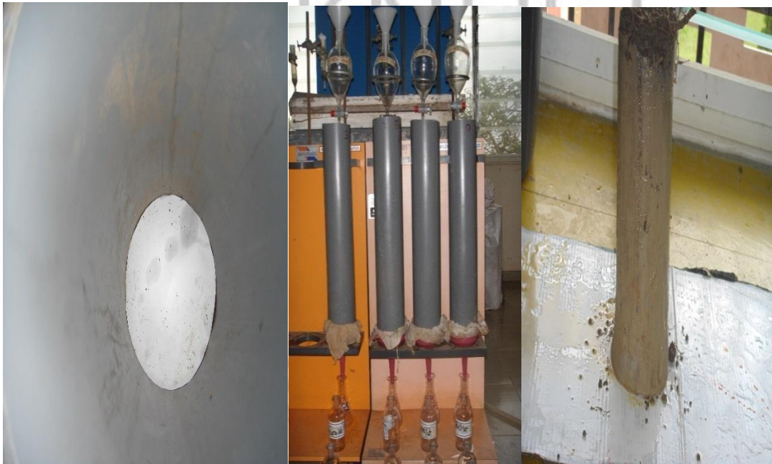
Plate 3: Inserted filter paper after spiking, leaching process and extruded soil after leaching.
