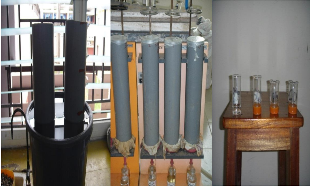
Plate 2: Saturation in artificial rain, equilibration and prepared \text{Cu}^{2+} solution for column spiking.
