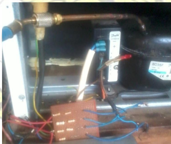
Figure 3.10: Resistors connected to the Electronic Control Unit of the VSDC Compressor
