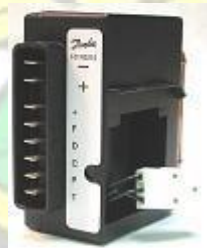
Figure 3.3: Electronic Control Unit for VSDC Compressor BD 35F
