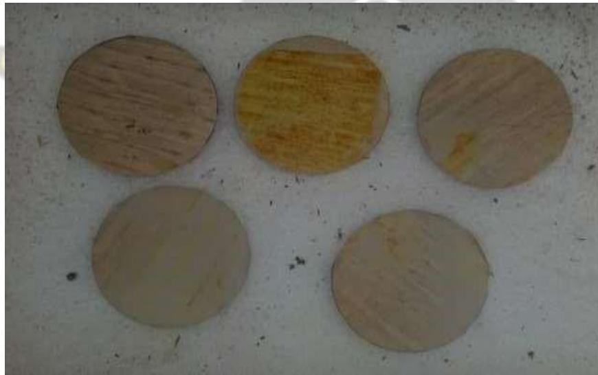
Figure 3.10 Samples made with plantain leaf Layer
