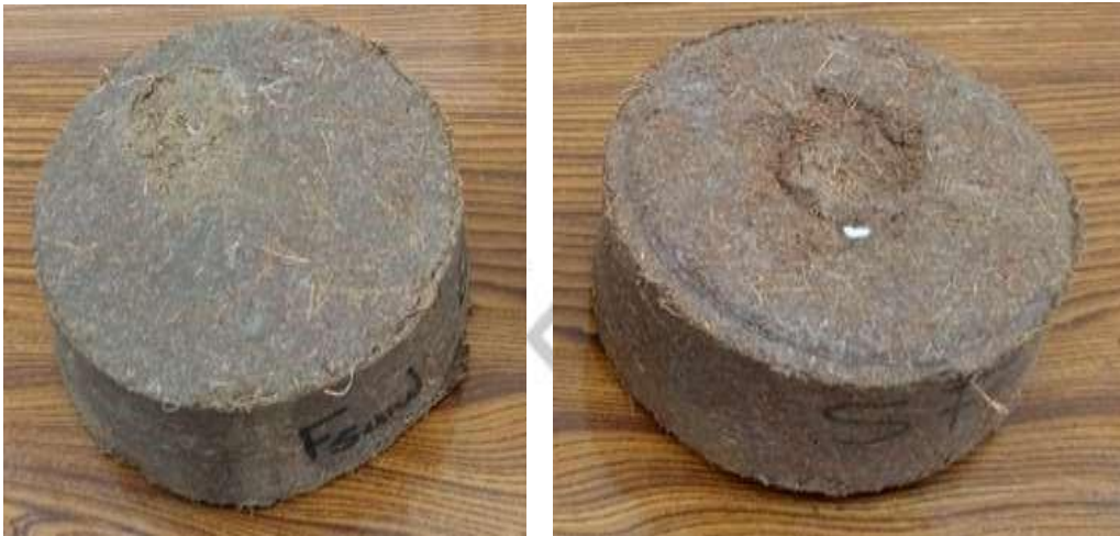
Figure 3.8 Fine grade sawdust ((k) with expansive clay and (l) without expansive clay)
