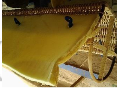
Plate 5.3h and 5.3i: Application of foam to the woven palanquin Source: studio work (2015)
