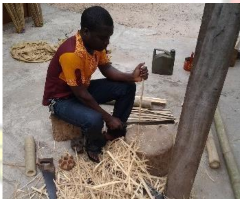
Plate 5.4c: Shaping the bamboo into ribs Source: studio work (2015)
