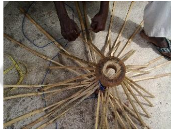
Plate 5.5a and 5b: Connecting nylon cord to the Ribs and the Runner (koboko) Source: studio work (2015)
