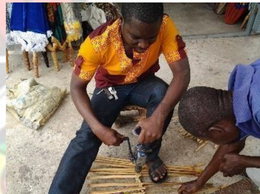
Plate 5.4d: drilling holes in the ribs Source: studio work (2015)
