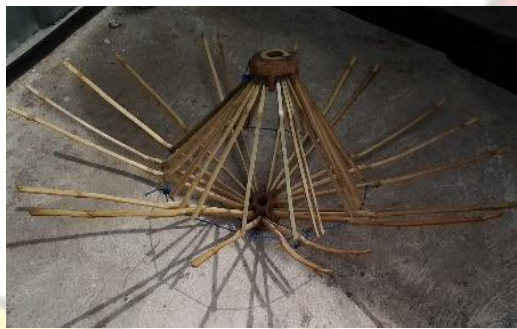
Plate 5.5d and 5e: Completed framework of the umbrella Source: studio work (2015)
