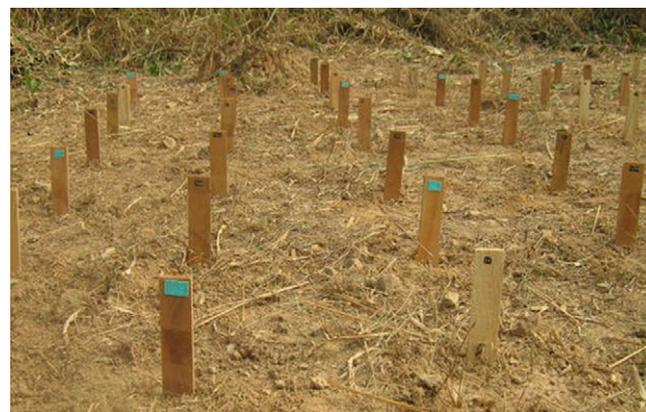
**Plate 1.** Freshly inserted *A. toxicaria* (treated and untreated) stakes at FRNR test-field.
