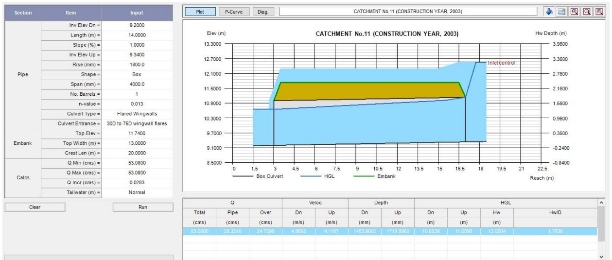
Appendix 4, Fig 4.82: Culvert at construction year 2003
