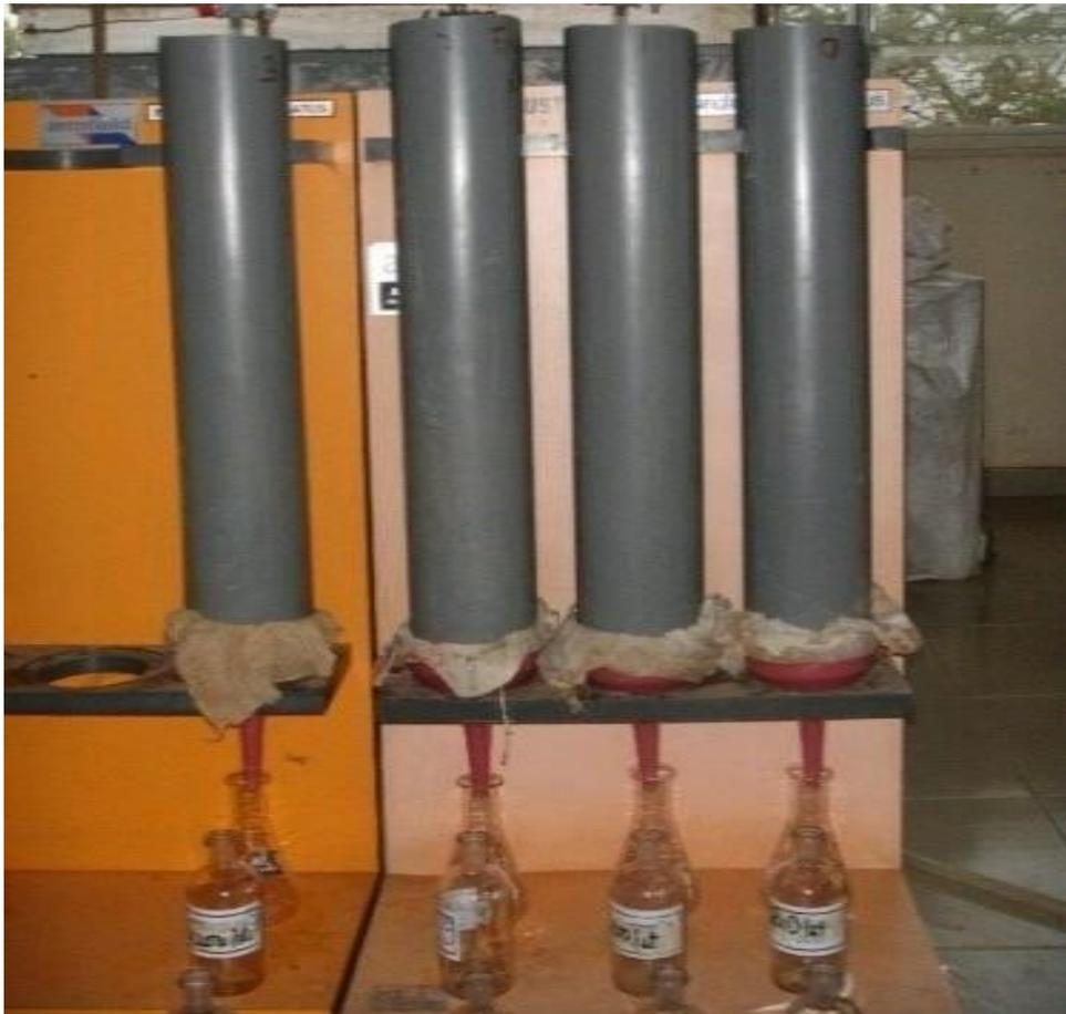
**Plate 2: Experimental setup for Pb transport.**
